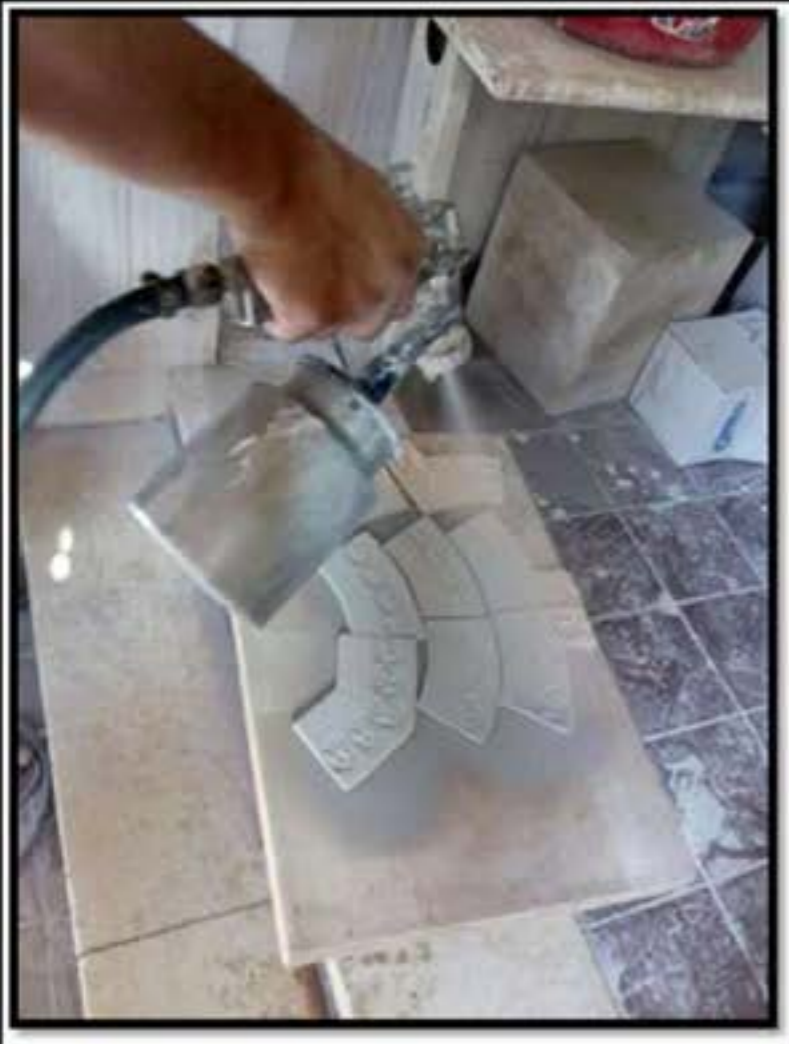
Spraying the glaze for the second firing
