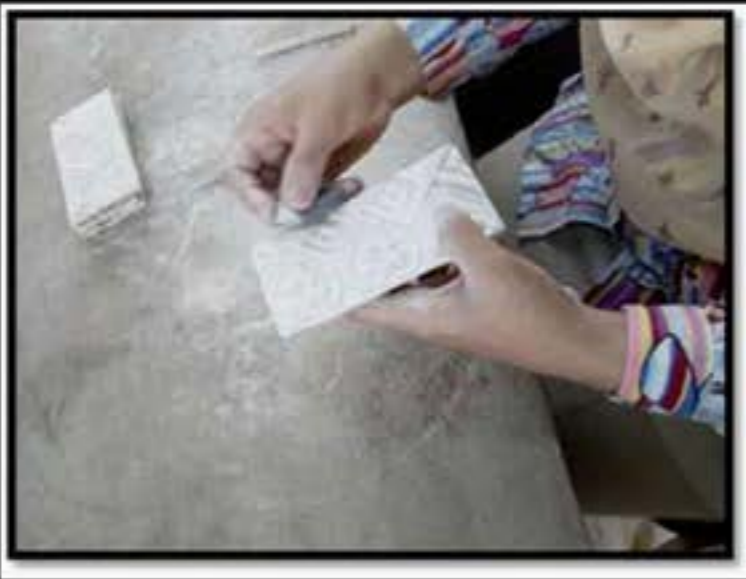
Sanding the tiles before first firing
